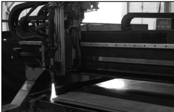
6" x 10' x 25' capacity flame cutting system
