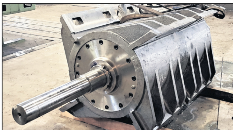
A crusher custom casting reverse engineered by Finch Manufacturing and Technology.
